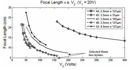
Figure 3: Focal Length versus. V<sub>2</sub>
