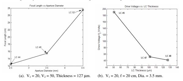
Figure 2. Relationship between aperture diameter, effective focal length, V2, and LC thickness
