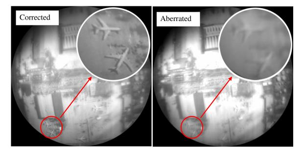
Figure 15: 25° Foveated Imaging,  $\lambda_C$  = 631  $\pm$  13 nm.
