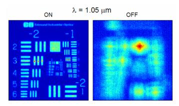
Figure 14: Resolution target images at 1.05µm with and without spectral correction
