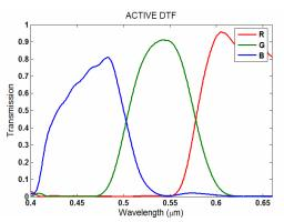
Figure 8: Digital Tunable Filter (DTF) pass-bands
