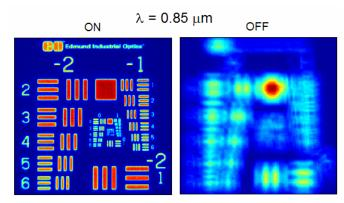
Figure 13: Resolution target images at the design wavelength (450nm), 650nm, and 850nm with and w/out correction
