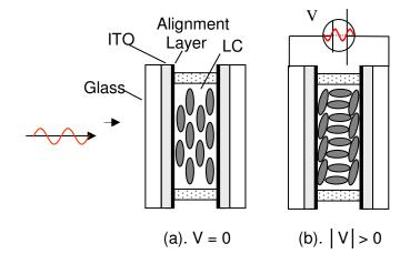
Figure 6: LC SLM Molecular Orientation
