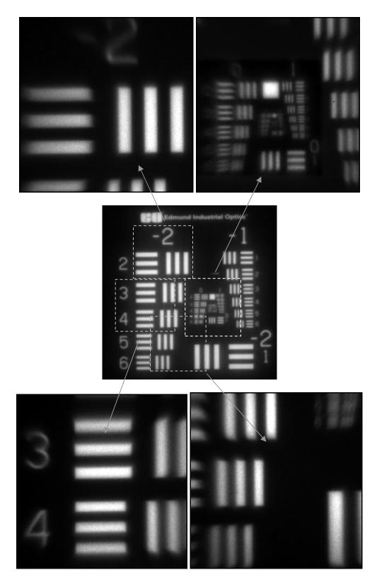
Figure 17: Off-Axis Magnification  $f_{EFF} = 105$  mm.
